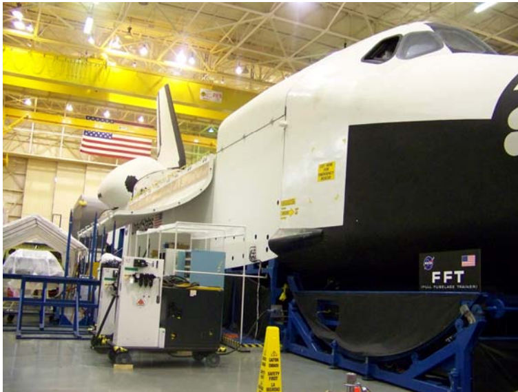
The Space Vehicle Mockup Facility, commonly known as Building 9 to NASA-JSC employees, contains a full-sized Space Shuttle trainer, without its wings which would occupy too much room.
